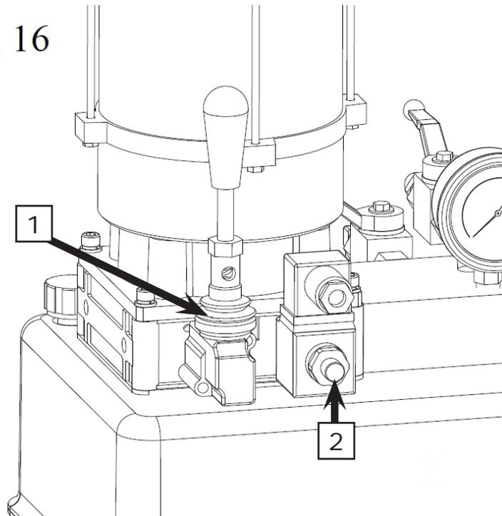
**Tip:** when a mechanical safety is released, it is advised to use a carton board to put between the safety pawl and the rack to avoid it from engaging. In this case, do not need to press the emergency button continuously. Screwing or loosing the screw can reduce or increase the lowering speed. After manual lowering of the lift, reset ordinary operating conditions. Lift cannot be lifted if solenoid valves are opened
