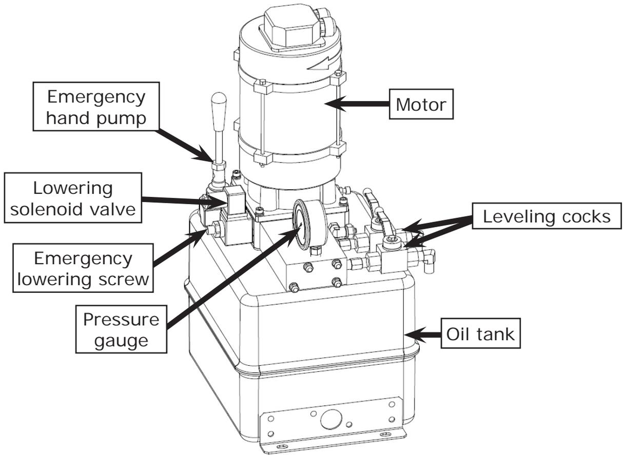
Figure 3 – Hydraulic Power Unit
