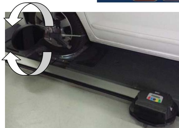
With the pin slightly braked, turn the target until you find the correct position.
