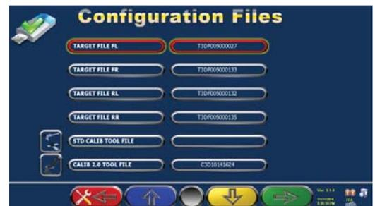
The Target files are located in the memory stick that came with the PC. Check on the memory key, in the "TARGET" folder, the files stored have the same name of the target mounted on Clamps. Connect the USB to the PC.
