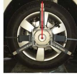
In the rear part of the Target, there is a label which identifies the working position.
