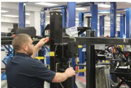
**Mechanical Lock & Lowering Valve Combination**
